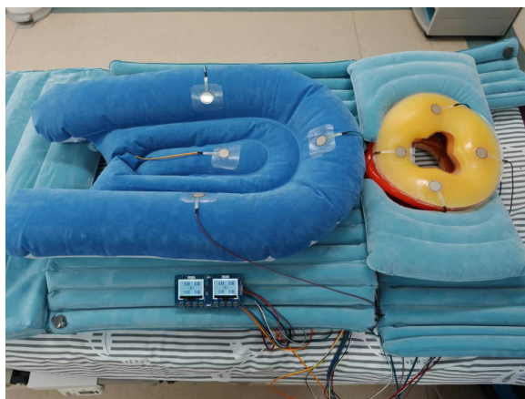
Fig. 1: Pressure sensing based airbag type prone position ventilation device
